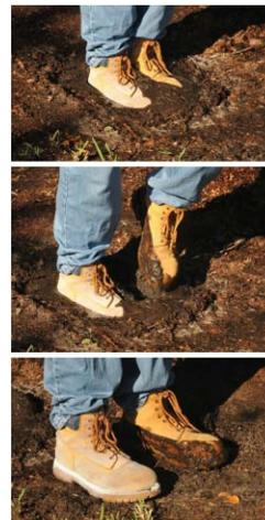
MUD TEST: Untreated boot (R) and boot sprayed with Ultra-Ever Dry (L).
