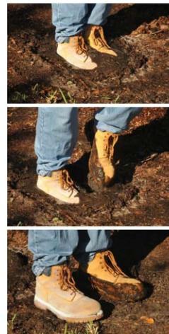
MUD TEST: Untreated boot (R) and boot sprayed with Ultra-Ever Dry (L).
